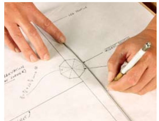
A full-size drawing. Use a flexible guide to fair the leg’s curve. Then draw the octagonal cross-section at the leg’s widest point. This view is used to size the eight sections that form the core.
